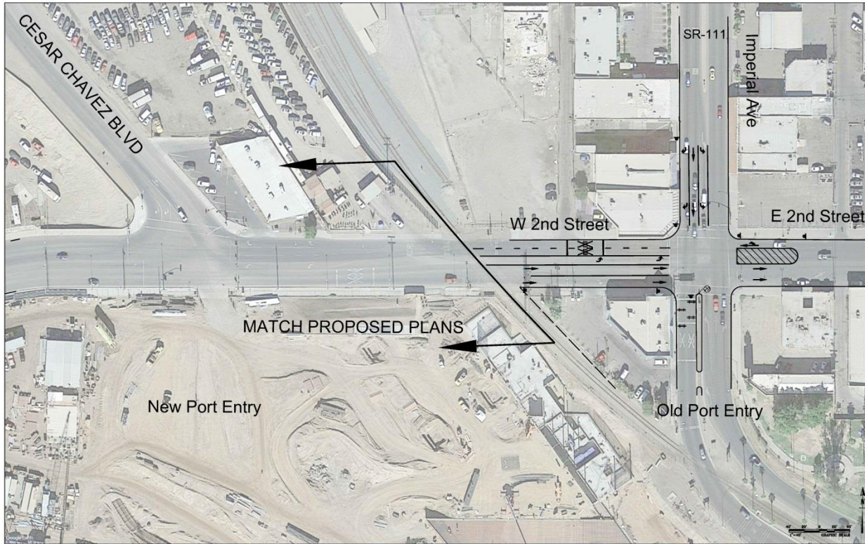
Figure 5.2 Lane Geometric Changes – Alternative 2A and 2B
