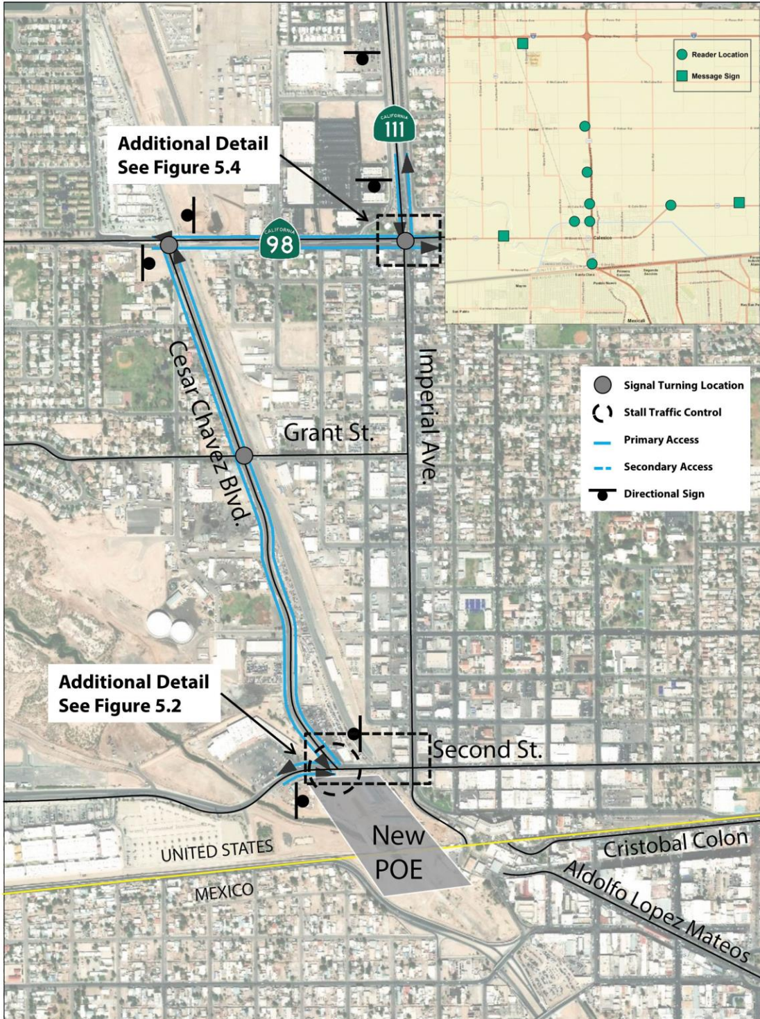
Figure 5.3 Traffic Control Plan – Scenario 2B
