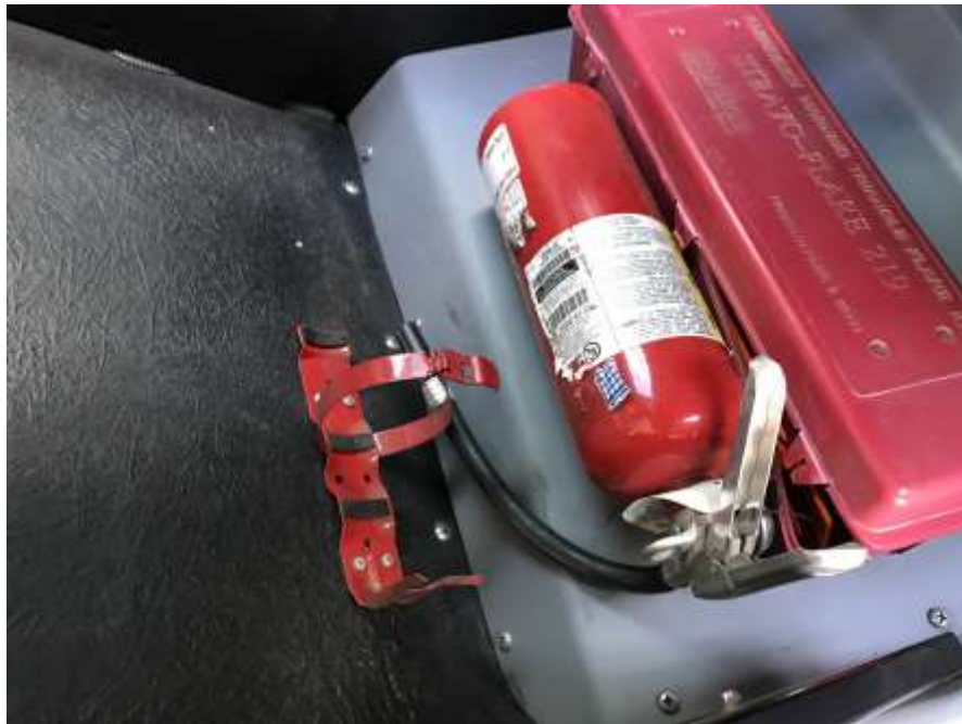
Bus 1201 – Fire extinguisher not secure
